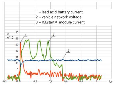
1. When starting the engine with the stock lead acid battery, the average discharge current of the battery is 230A, the average voltage in the vehicle network is 9V, start time is 0.68s.
